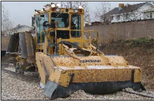
Rail Sweeper and Salvage
