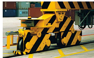
RMG Crane Steel Wheel Trolley
