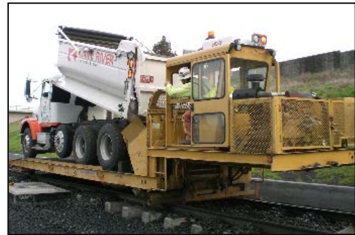
Flat-bed or Bucket Rail Transport
