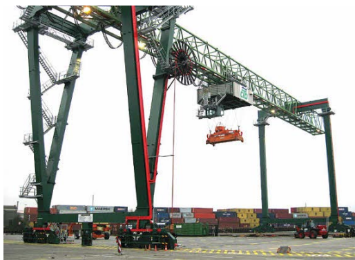
Rail Mounted Gantry Crane (RMG)
