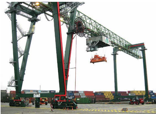
Rail Mounted Gantry Crane (RMG)
