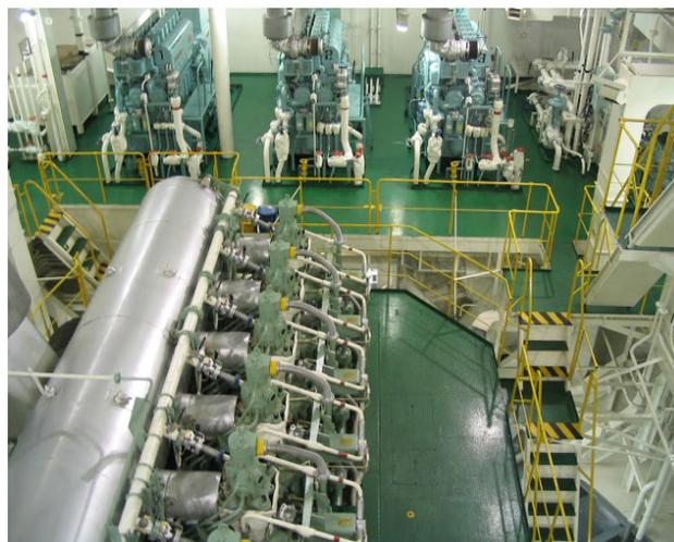
Passenger cruise vessels, and some tankers, use a configuration that is referred to as diesel-electric. These vessels use large diesel generator sets to provide electrical power for both propulsion and ship-board electricity.
