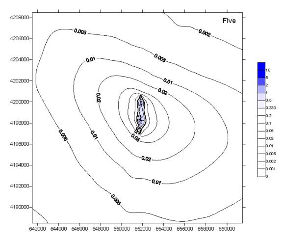
Figure 9. AERMOD's Simulated Diesel PM Concentrations (due to Onsite and Off-site Diesel PM Emissions) around UP Stockton Railyard Using Five-year Meteorological Data.
