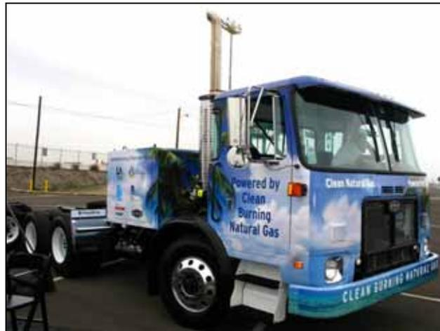
The CNG HD port drayage truck project proponents ultimately hope to transition the CNG drayage truck technology to a CNG/hydrogen fuel blend technology. Project proponents believe a CNG/hydrogen fuel blend may be able to provide an additional 30 to 50 percent in NOx emissions reductions.
