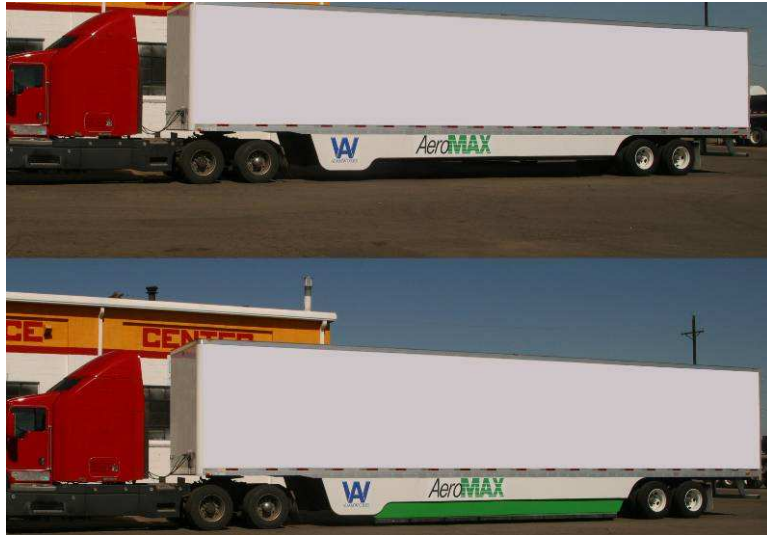
Figure IX-3: Adamworks Aeromax Retractable Fairing
