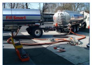
Fuel Transfer From Cargo Tank to UST Volume Meter Installed on Vapor Return
