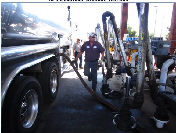
Figure 9: Bottom Loading of Cargo Tank Prior to Efficiency Testing At the Morrison Brothers Test Site
