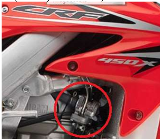
Figure V-10: Air Injection System (Courtesy of Dirt Action)
