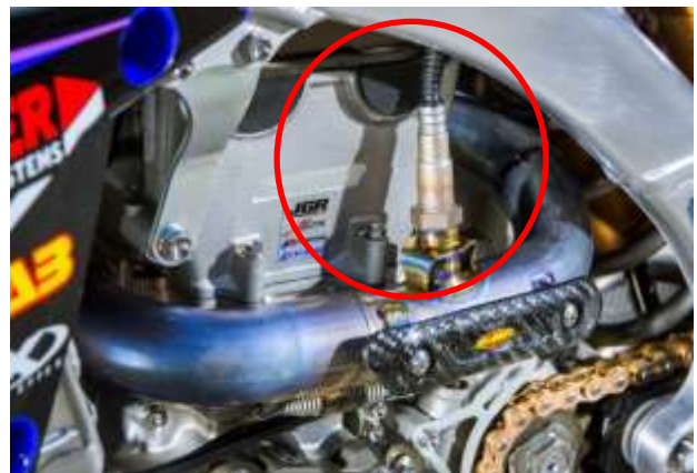
Figure V-12: Oxygen Sensor (Courtesy of Transworld)
