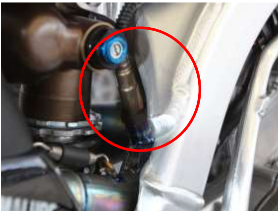
Figure V-11: Oxygen Sensor (Courtesy of Grind TV)
