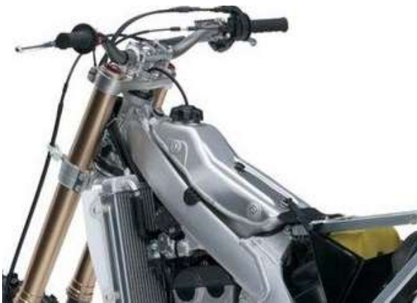
Figure V-14: 2014 Suzuki RMZ450 OE Aluminum Fuel Tank (Courtesy of TopSpeed)
