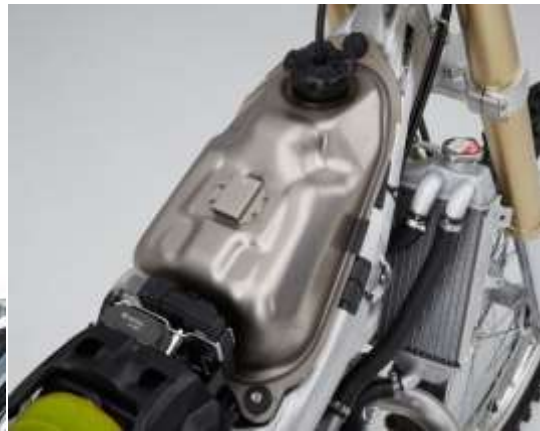
Figure V-15: 2017 Honda CRF450R OE Titanium Fuel Tank (Courtesy of Cycle World)
