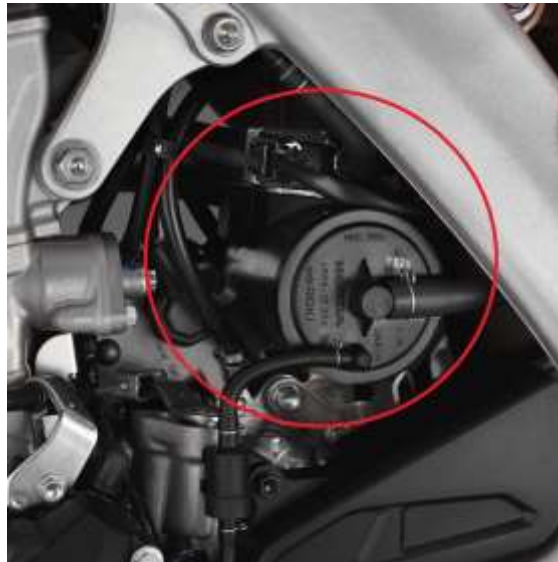
Figure V-16: 2019 Honda CRF450X OE Carbon Canister System (Courtesy of Ultimate Motorcycling)
