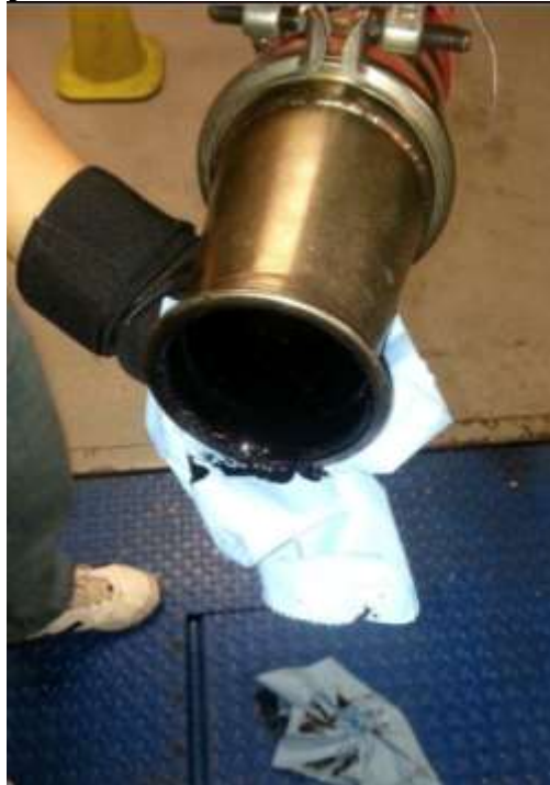
Figure II-7: Oily Residue from Two-Stroke Motorcycle Exhaust
