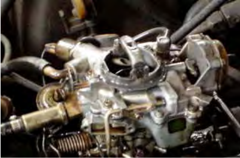
Figure 4-4. Carburetor Cleaned With Alternative Cleaners
