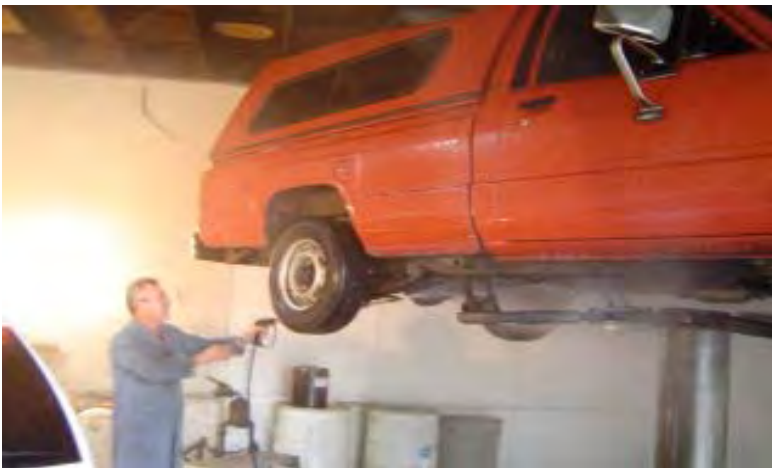
Figure 4-3. Detailer Cleaning Undercarriage of Truck
