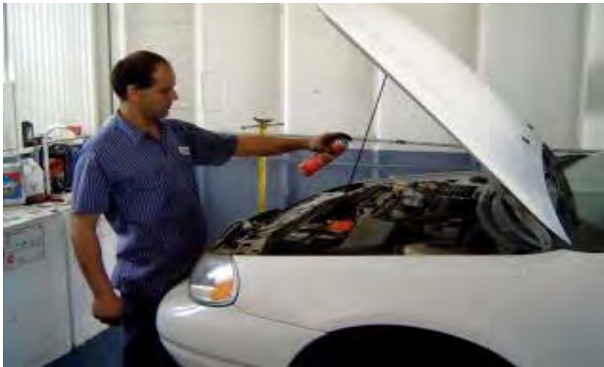
Figure 4-5. Technician Performing General Purpose Degreasing
