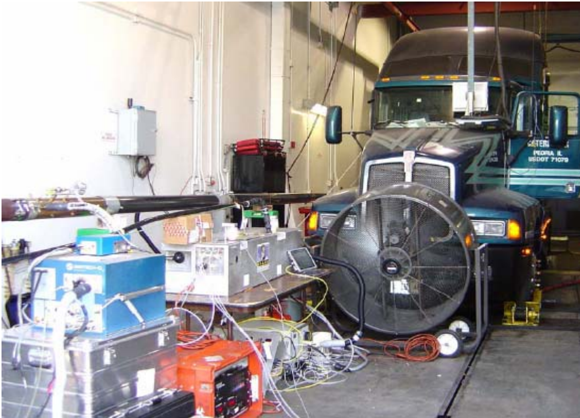
Figure 2-6. Experimental Set-up for the Chassis Dynamometer Testing
