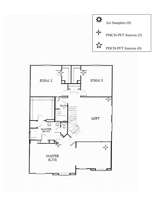
Figure 12. Floor plan of P3 second floor, depicting the locations of the PFT sources.
