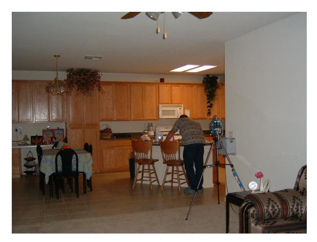
Figure 1. Pilot Home P3, photograph of air sampling rig in the family room.
