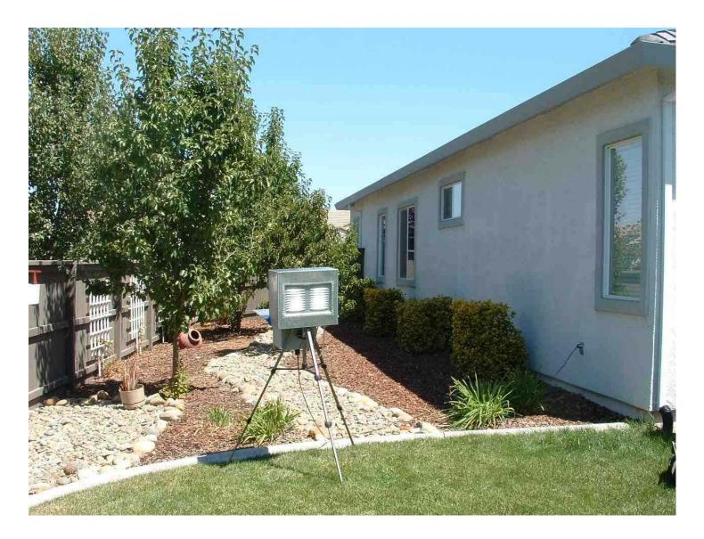
Figure 2. Outdoor air sampler for formaldehyde, VOCs, PM<sub>2.5</sub>, NO<sub>2</sub>, CO, CO<sub>2</sub>, temperature, and relative humidity, with outdoor radiation/rain shield.
