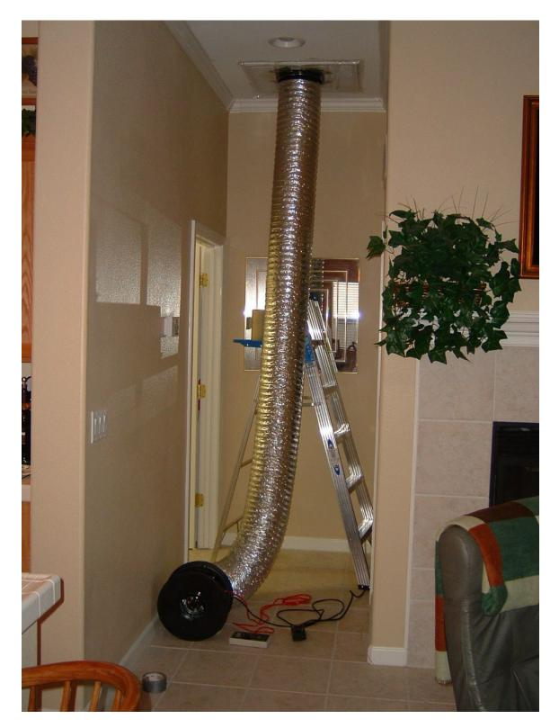
Figure 4. Pilot Home P2, Duct Blaster installed at return air inlet of forced air heating/cooling system.
