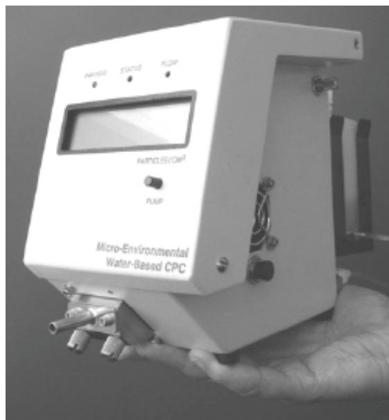
Figure 1.2. Photograph of the Micro-Environmental Water-Based Condensation Particle Counter (ME-WCPC) (Hering, 2006).
