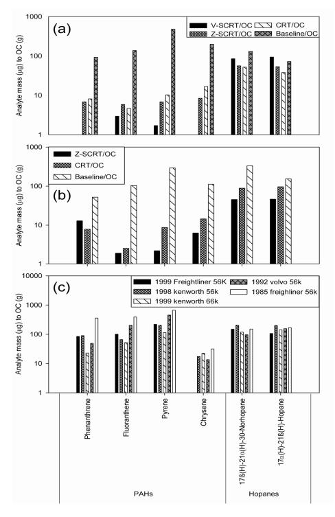
Figure 5-5 Comparison of the ratios of PAHs, hopanes and steranes to organic carbon emission factors in  $\mu g/g$  from baseline and controlled vehicles. (a) running on UDDS cycle. (b) cruise cycle. (c) Ratios of PAHs, hopanes and steranes to organic carbon emission factors in  $\mu g/g$  as reported by Riddle et al., (2007)
