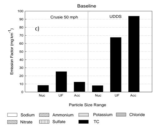
Figure 5-6 Emission rates of size-resolved PM chemical species. a) Cruise 50 mph, b) Transient UDDS c) Baseline vehicle.
