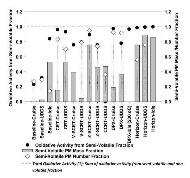
Figure 6-2 Relationship between oxidative activity and semi-volatile PM fraction at 150°C.
