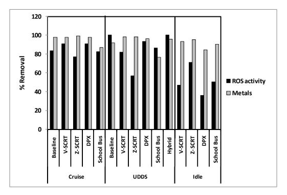
Figure 6-5 Percent removal of ROS activity in relation to that of aggregate water soluble metals after Chelex treatment of the exhaust PM samples from test vehicle-configurations under different driving cycles.
