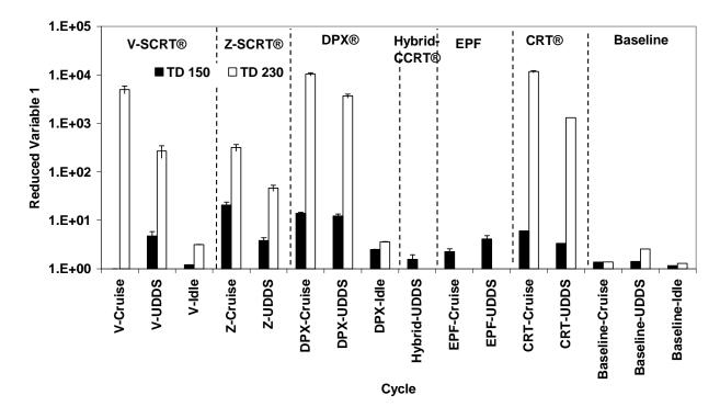
Figure 4-3 Reduced Variable 1 (R): Ratio of total particle to solid or thermo-denuded particle count.
