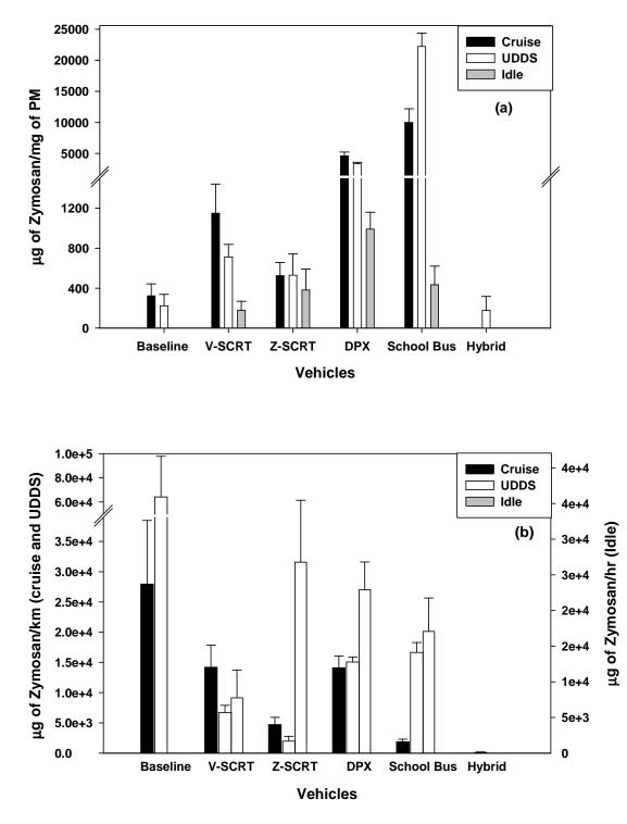
Figure 6-4 Reactive Oxygen Species (ROS) activity of PM from the tested vehicles, expressed as (a) per mass of PM, and (b) per km (or hr for idle) of vehicle driven.
