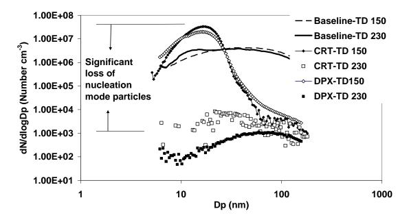
Figure 4-4 Size distribution of thermo denuded aerosols for cruise mode.
