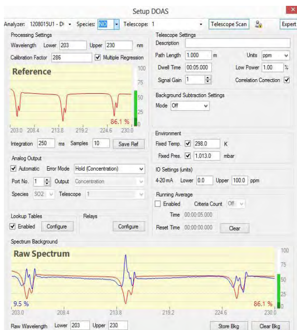
Figure 5-4. Shows initial DOAS configuration file and reference spectra for NO, notice strong NO absorption from 214 nm to 216 nm.
