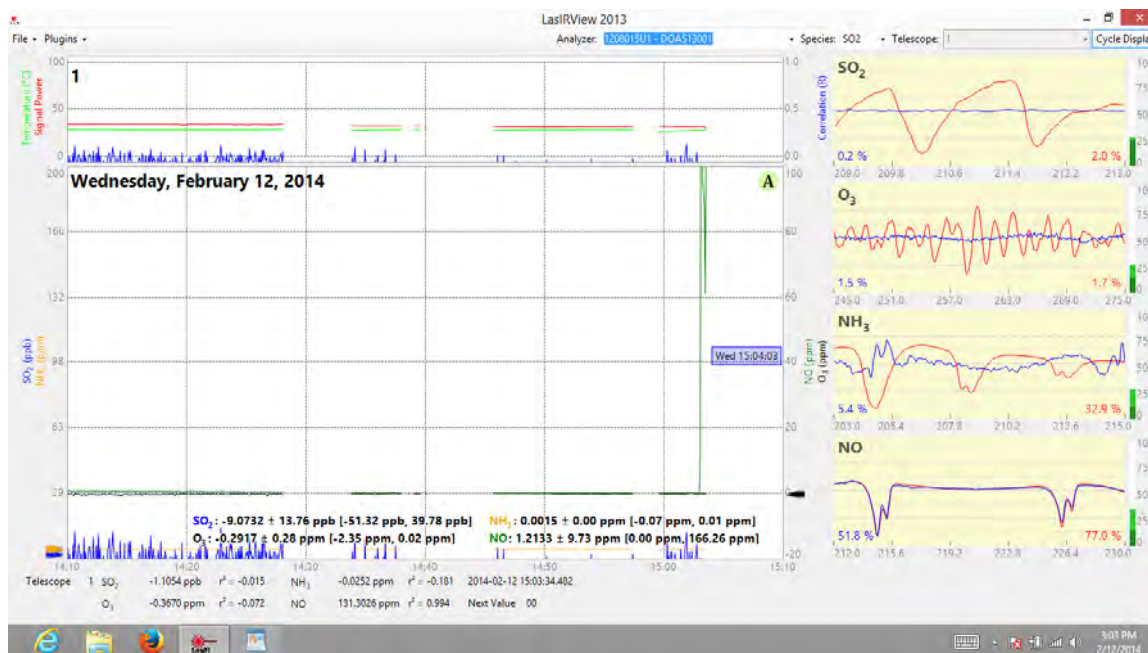
Figure 5-15: Diesel test at engine turn on, note there is no detectable SO 2 (-1.105 ppbV).
