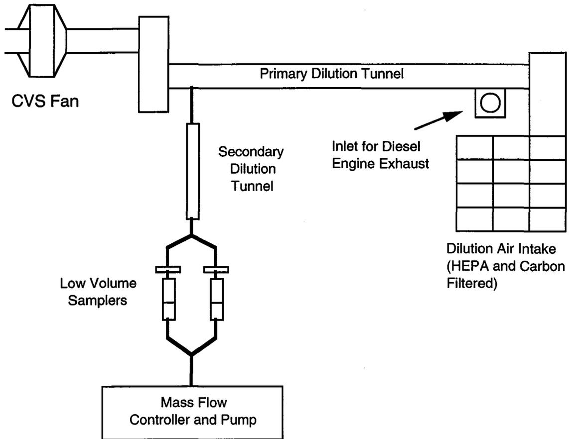
Figure 2. Dilution Tunnel for Heavy-Duty Diesel Exhaust and Sampler at the LACMTA Facility.
