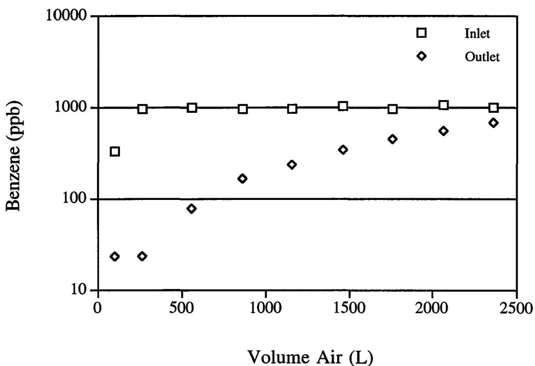
Many of the toxic compounds to be trapped have considerably lower vapor pressures than benzene and therefore would have significantly higher breakthrough volumes. The breakthrough volume of benzene provides a lower limit volume of gas that can be sampled before the sorbent module should be changed. The sampling system, as designed, appeared to be efficient for collecting the semi-volatile compounds anticipated to be present in the vapor-phase of diesel engine exhaust.
