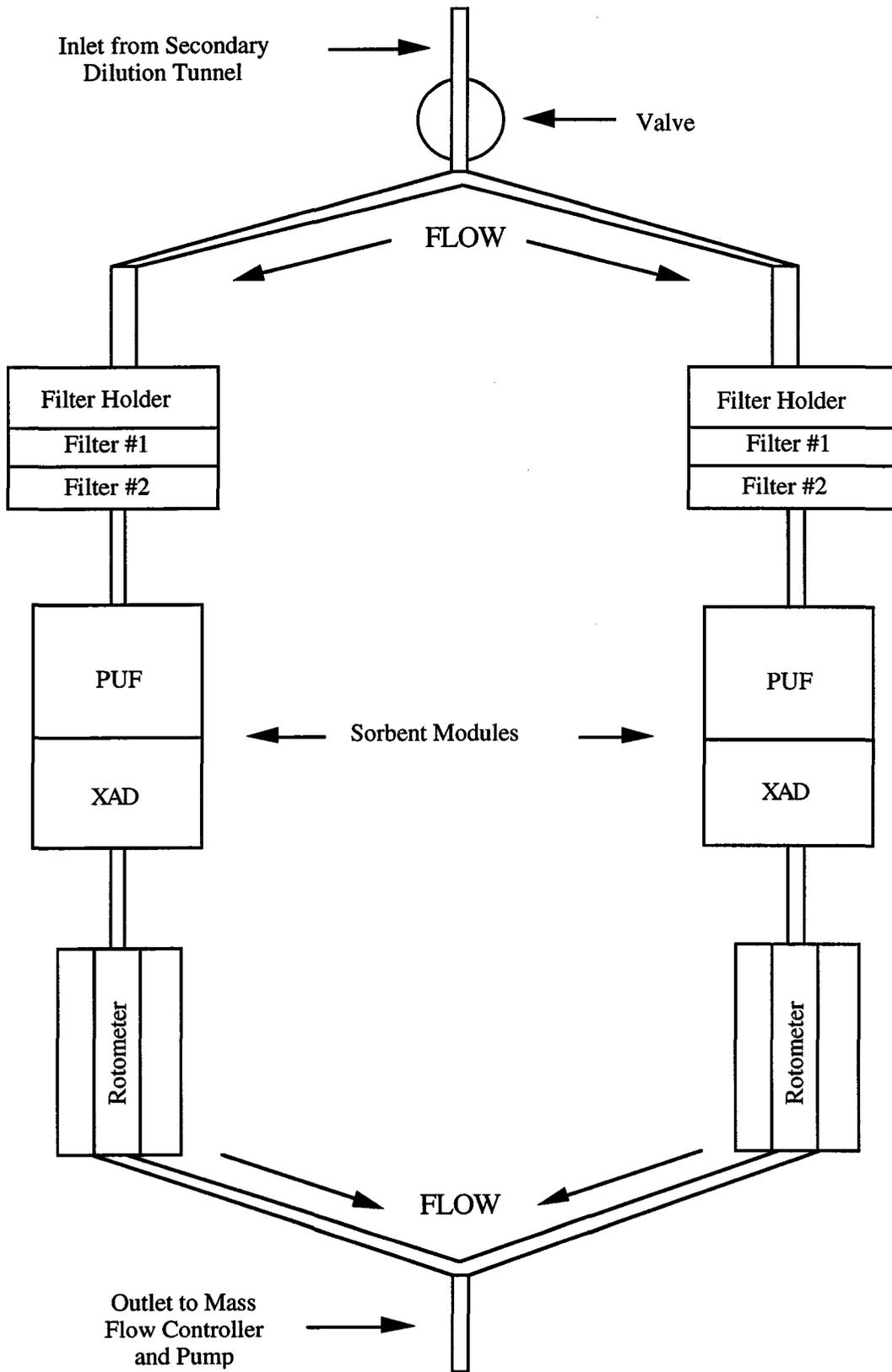
Figure 1. Particulate and Vapor-Phase Sampler.
