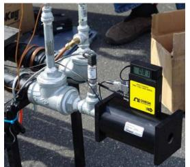
Figure 24: Flow, temperature, & pressure sensors mounted at expansion pipe outlet
