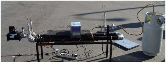
Figure 23: Emissions Test Equipment Setup
