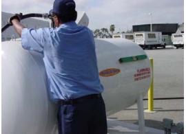
Figure 21: Operator Filling Tank with Maximus™ Shown to Tank Attached during Most Recent Field Tests
