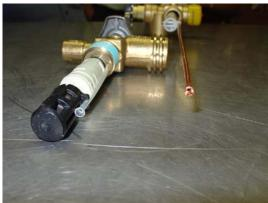
Figure 1: Outage Gauge (FMLLG) Dip Tube Internals
