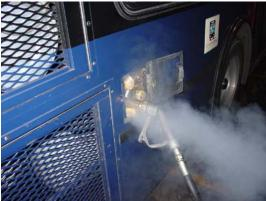
Figure 2: LP Gas Emissions from Bus Tank Outage Gauge
