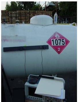
Figure 12: Field Tests of Beta-Prototype Maximus™ SFI Incorporating New Sensing Methods
