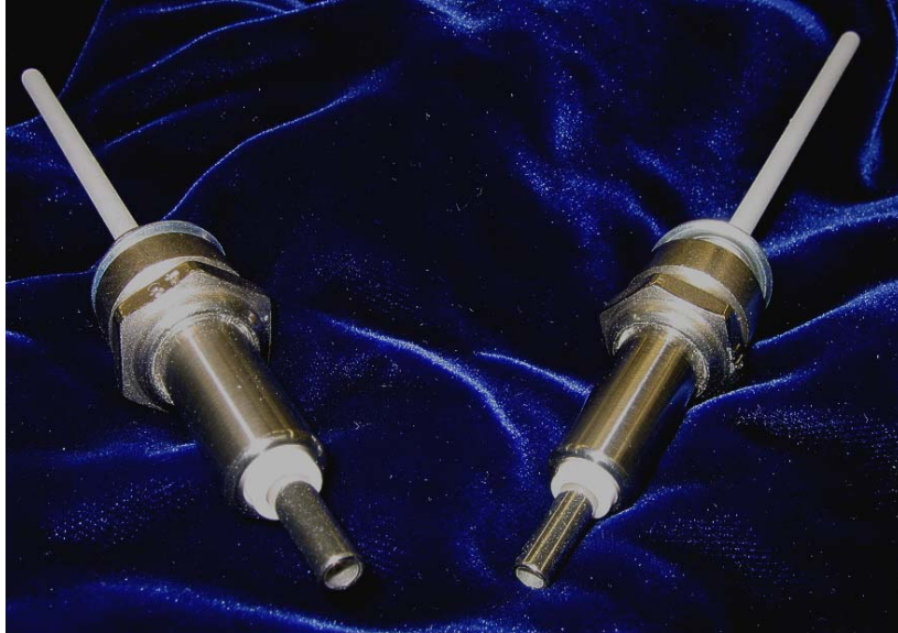
Figure 4-1. Shielded version of PM sensor
