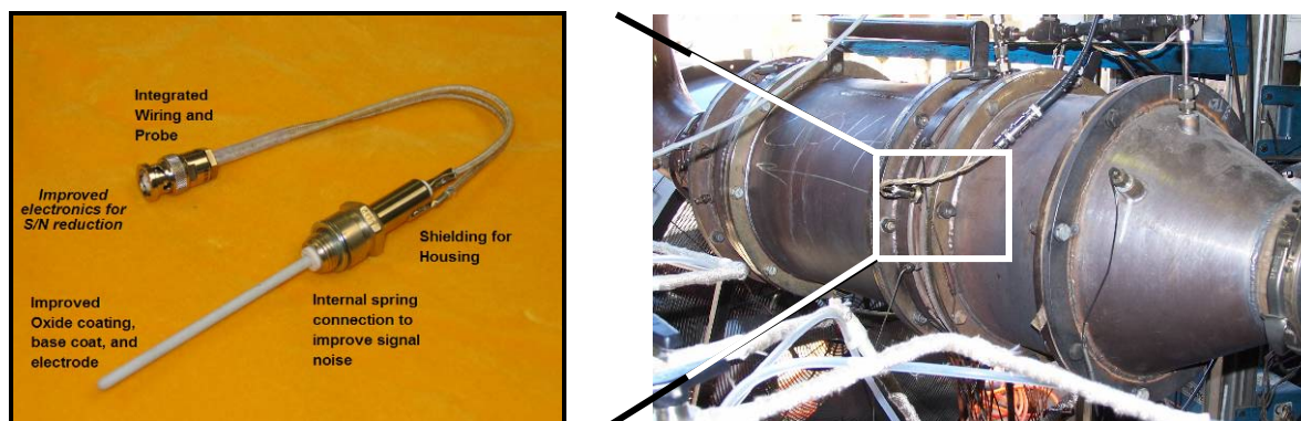
Figure 2-1. (a) PM sensor (left) (b) Sensor installed in the pre-DPF environment (right)
