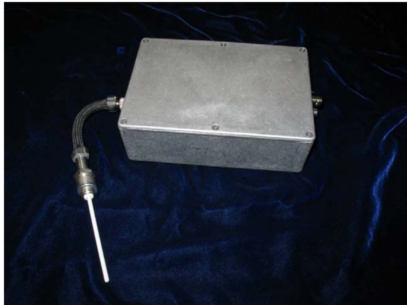
Figure 4-3. PM sensor with associated electronics
