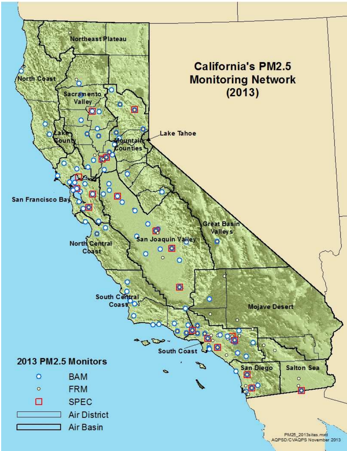
Figure 1: PM2.5 Monitoring Stations in California
