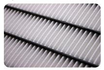
MERV 9 to 12 rating. They cost about \$10 to \$20 for disposable one-inch models. Before using a filter rated MERV 9 or higher, you may want to have an HVAC technician check your central system to be sure it can handle any added airflow resistance that higher efficiency filters may cause. Some higher efficiency filters are designed to avoid excessive airflow reduction (e.g. the filter is highly pleated, or has deeper pleats), so you may want to use one of those.
