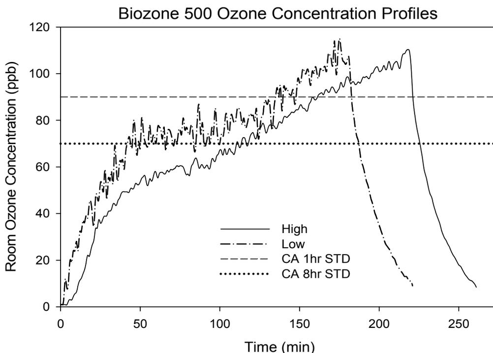
**Figure 6. Ozone Concentration Profiles for Unit 2 Room Tests**
