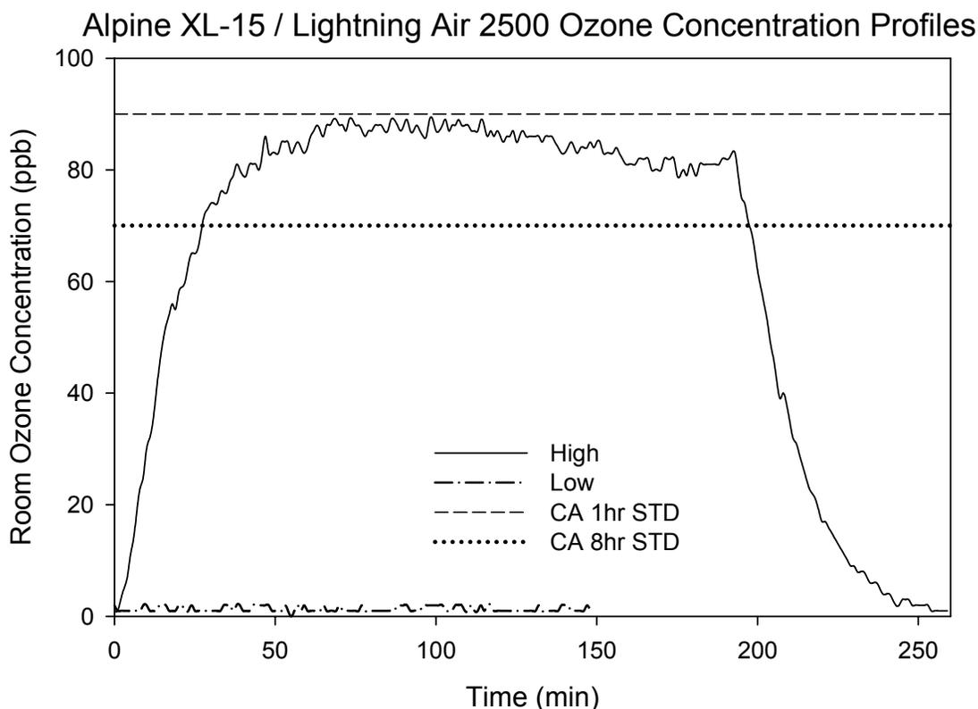
**Figure 5. Ozone Concentration Profiles for Unit 1 Room Tests**
