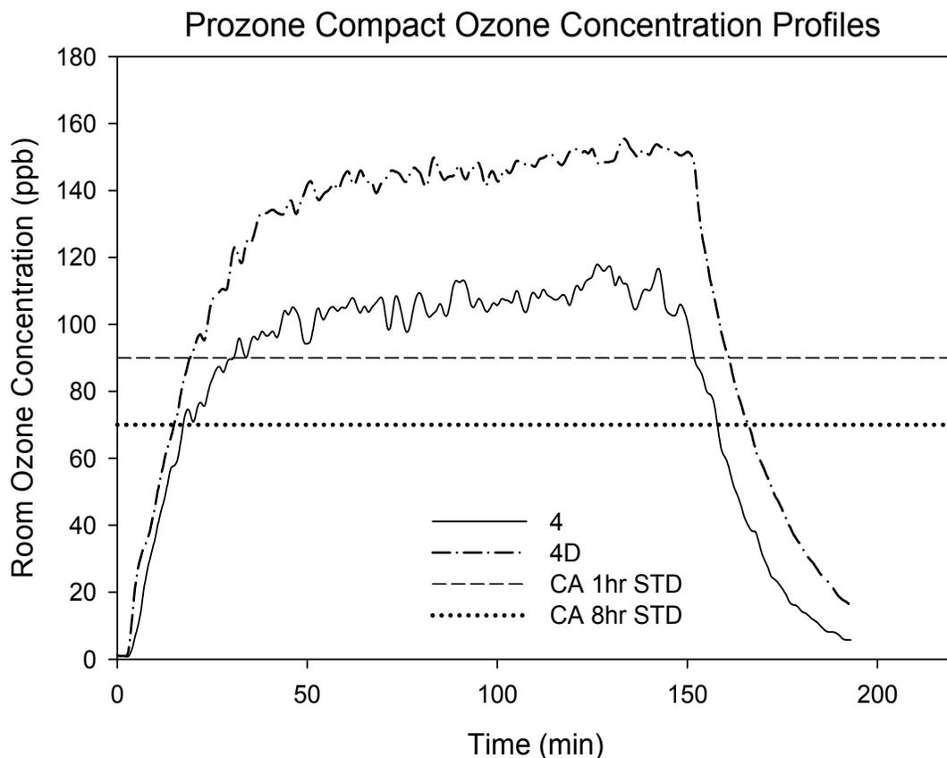
Figure 8. Ozone Concentration Profiles for Unit 4 Room Tests
