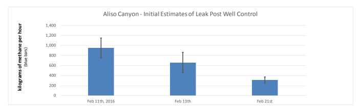
Once the off gassing is no longer affecting the overall emissions of the site, the measured emission rate should flatten out and stay constant.
