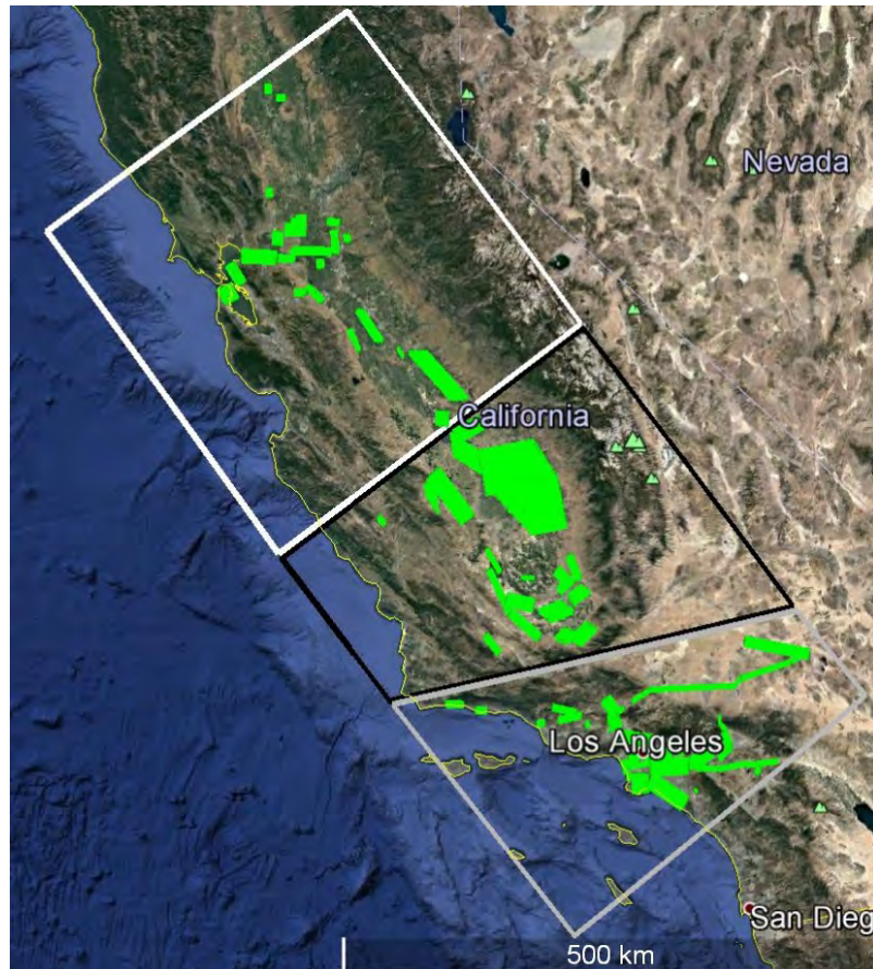
Figure 4-1 As-flown flight lines (green) for AVIRIS-NG Fall 2016 survey. The coverage of the completed lines is not identical to the boxes shown in Figure 3-6 due to modifications to the initial flight plan and the addition of two mini-intensive flight campaigns to map high pressure natural gas transmission lines in the LA Basin and an area near Visalia. Regional
