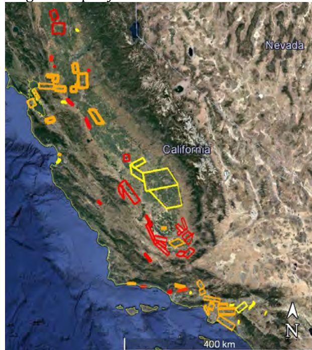
Figure 3-6. AVIRIS-NG flight boxes for Fall 2016 campaign surveying the energy sector (red), non-energy sector (yellow), and mixture of these categories (orange).
