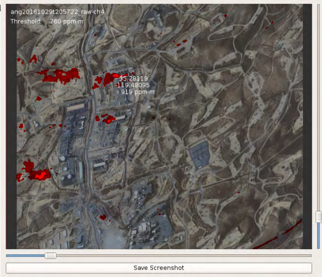
Figure 3-4. Real time methane mapping onboard the aircraft. Red methane plumes are overlaid on raw AVIRIS-NG images with estimated peak enhancement (ppm-m) and plume source coordinates.
