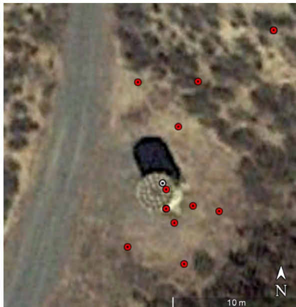
Figure 3-11. Example of methane source attributed to a vent stack at the Honor Rancho gas storage facility. The red markers indicate the detection of multiple plumes over several weeks that were used to infer the existence of the source (white marker centered on vent stack).
