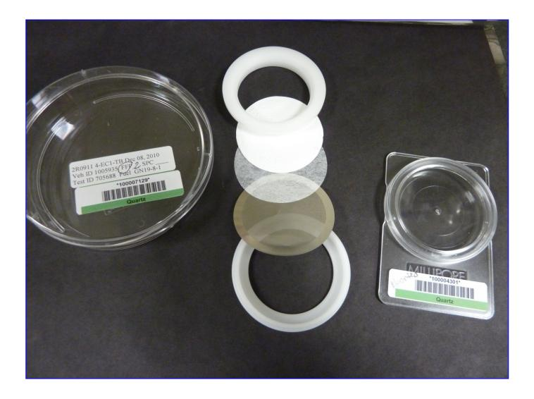
Figure 5: Quartz filter assembly
