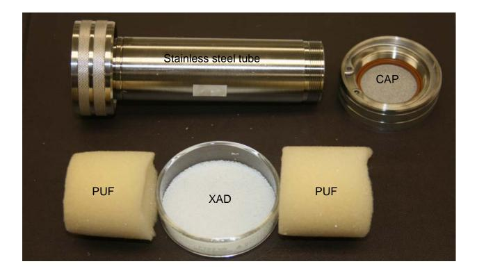
Figure 7: Sampling media holder for the collection of the semi-volatile PAHs
