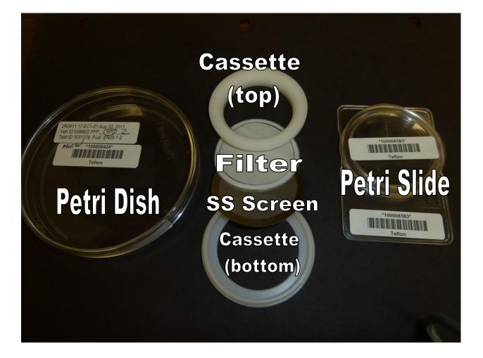
Figure 4: Teflon filter assembly
