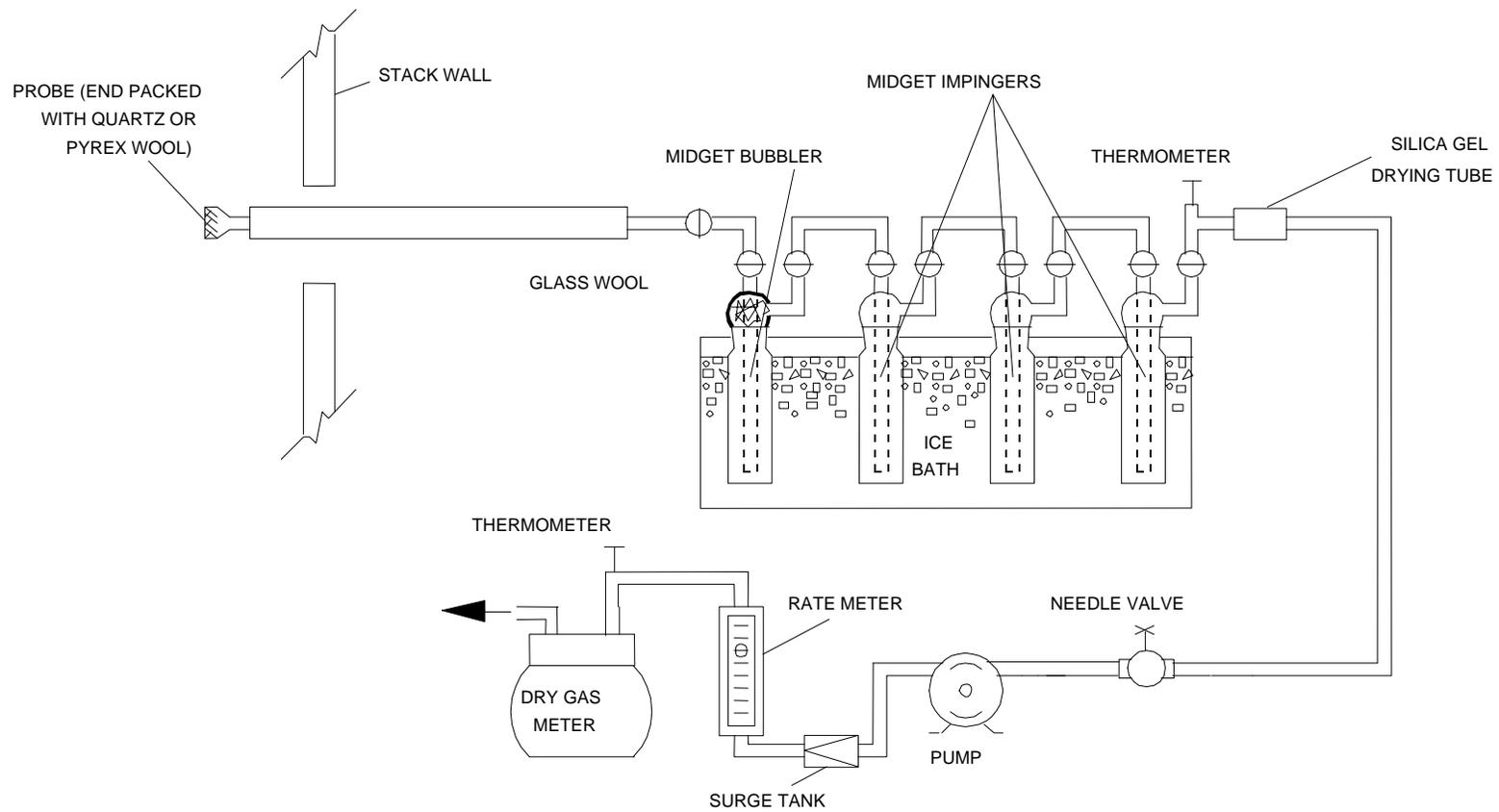
Figure 6-1. SO<sub>2</sub> Sampling Train
