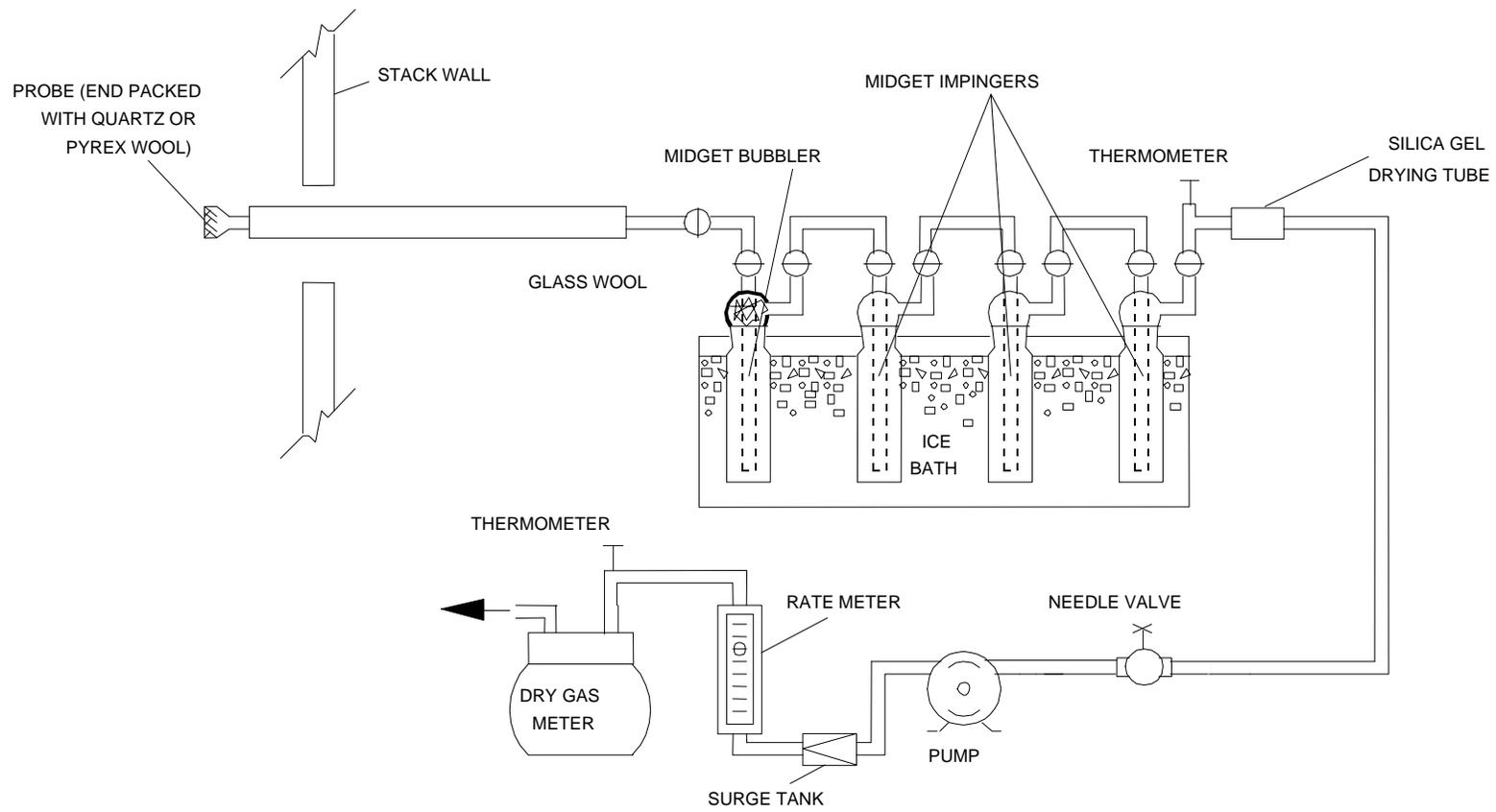
Figure 6-1. SO<sub>2</sub> Sampling Train
