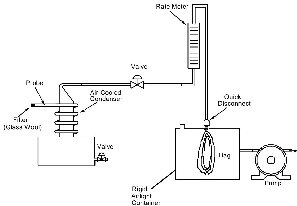
**Figure 10-2 Integrated Sampling Train**
