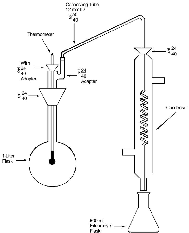
**Figure 13A-2. Fluoride Distillation Apparatus.**
