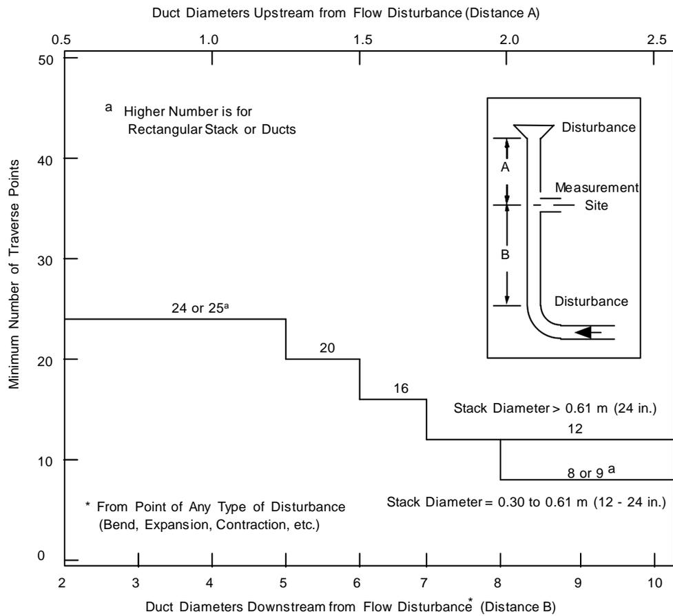
Figure 104-3. Minimum number of traverse points for particulate traverses.
