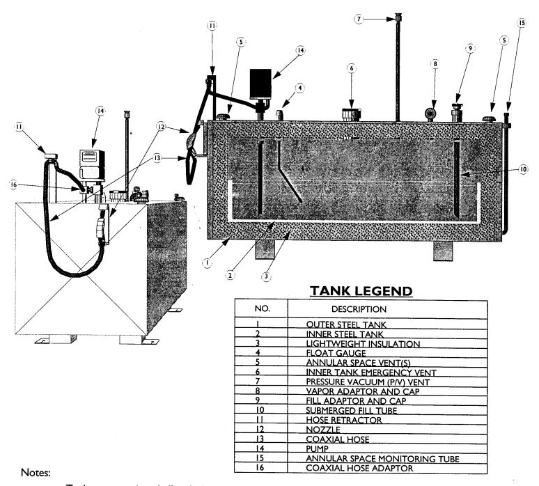
Tank construction shall include a minimum of 6 inches of proprietary insulating material between the interior holding tank and the exterior containment tank.
