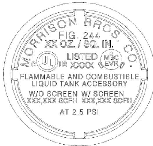
Figure 1A-2 Morrison Bros. 244 Cover Marking Diagram (The X designation will contain a value which may vary depending upon the size and pressure setting of the vent)
