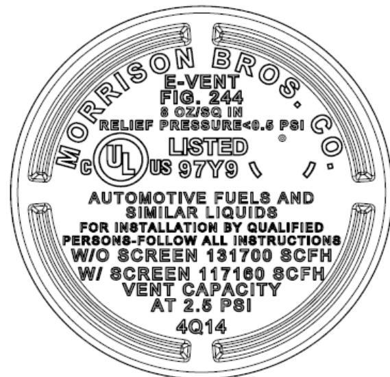
Vent sample with relief opening pressure less than 0.5 psi.
