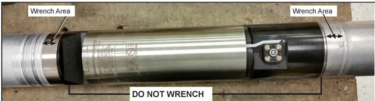
Figure 11: Do Not Tighten on the Float Shield
