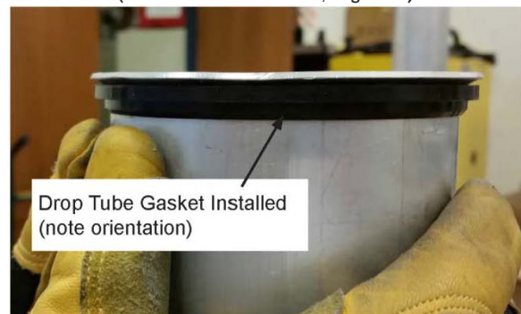
Figure 7: Drop Tube Gasket Installed
